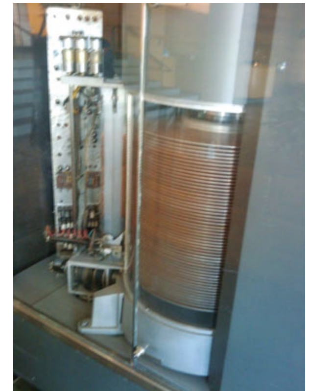
One of the first commercial disk drives from IBM. It has a 5 MB capacity and it's stored in a cabinet roughly the size of a luxury refrigerator. In contrast, a 32 GB microSD card measures around 5/8 x 3/8 inch and weighs about 0.5 gram.
